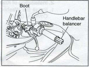
2. Remove the lever pivot bolt and nut. (LH and RH)
