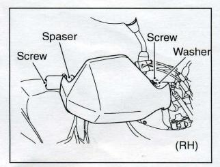
8. Install the Washer © and tighten the nut.
